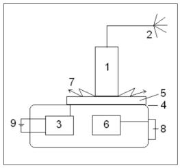
Figure 1. The schematic design of the "Eco-Tester" Electrophotonic Sensor. 1 – titanium cylinder; 2 – special antenna; 3 – impulse generator; 4 – transparent conductive layer; 5 – quartz electrode; 6 – TV system; 7 – gaseous discharge; 8 – memory stick; 9 – 12 V rechargeable batteries.
